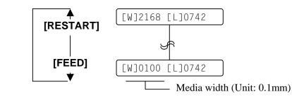
**[FEED]** key: Pressing the **[FEED]** key one time causes a -1 change, up to 100.
